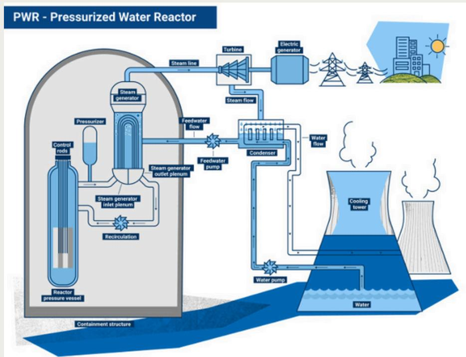
Fig 1. Schematic of a pressurized water reactor (PWR) [2]
